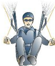
Lowering the control handles to decrease airspeed
